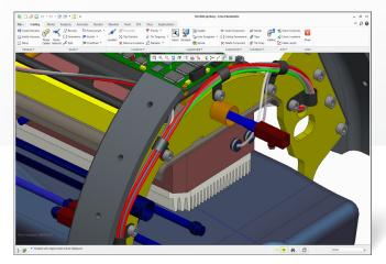
Automated cabling design capabilities make it easy to move components and connectors without manually rerouting wires and cables.
