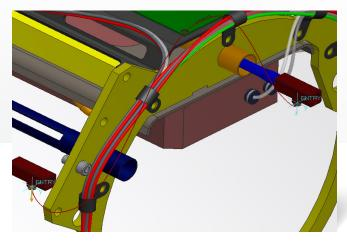
Determine the connections either manually or from logical information. Creo PCX automatically generates a simple path which then enables the user to find the optimum path faster.
