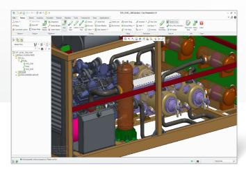
With Creo PCX, you can immediately determine the best piping routes between even the most complex systems.
